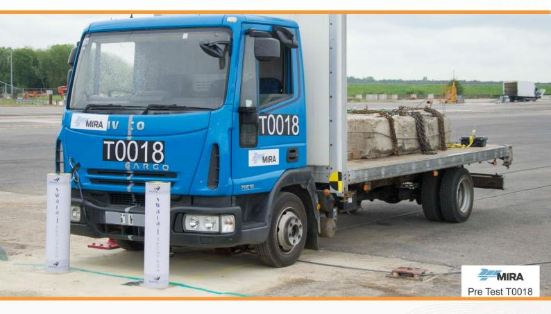
Swaraj Secutech presents India's first manufactured and physically crash tested indigenously designed bollard. Our bollards have been impact tested by Horiba, MIRA. U.K. wherein the bollard was hit at 48 km/h by a fully laden 7.2-ton truck and achieved a penetration of only 0.1 m.
